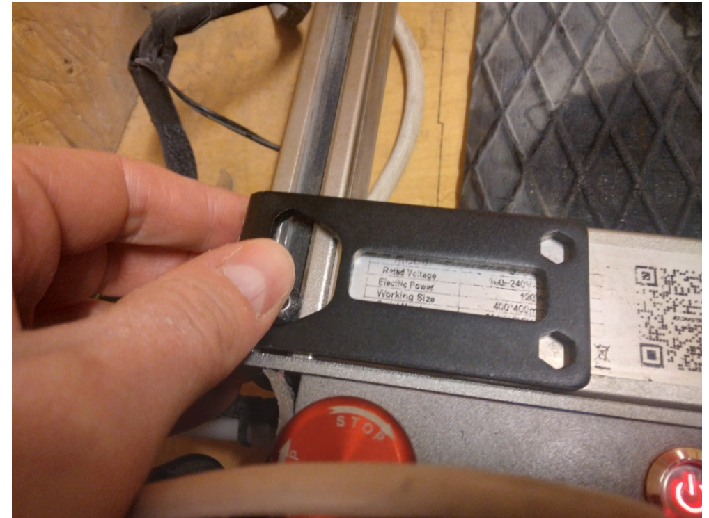
Figure 27: Place the spacer back in its proper place
