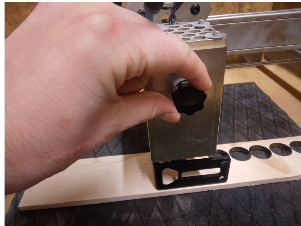
Figure 25: Tighten up the laser again by turning its screw
